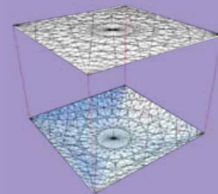
**DRAWING OF THE SUPPORTING STRUCTURE OF THE ROOF AT THE NETHERLANDS MARITIME MUSEUM IN PLAN. BELOW THE CURVED VERSION ACCORDING TO THE HANGING CHAIN PRINCIPLE**
