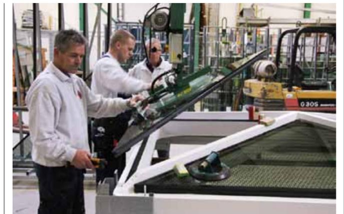
THE CUPOLAS ARE GLAZED WITH TRIANGULAR GLASS PANELS MADE BY SCHEUTEN GLAS IN HOORN.
